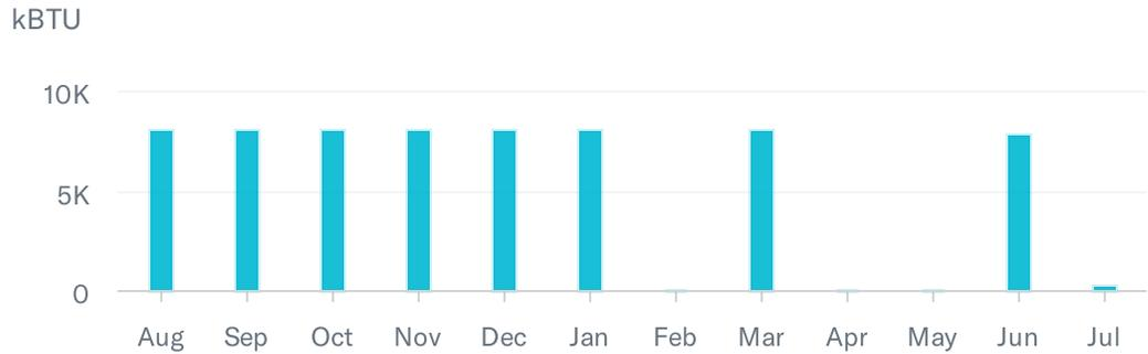
**Source Energy** represents the total energy used by the building, including energy consumed in extraction, processing and transport of primary fuels such as coal, oil and natural gas; energy losses in thermal combustion in power generation plants; and energy losses in transmission and distribution.
